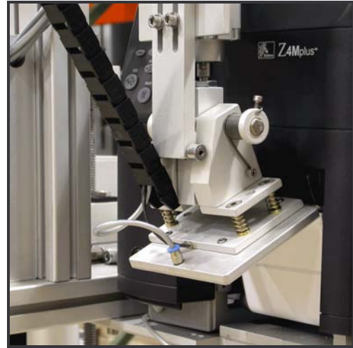
The tamp pad should be aligned with the peel edge.
