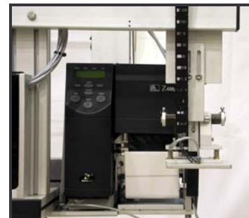
The tamp should be vertically aligned with the peel edge of the printer.
