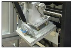
Tamp / Blow Alternative-For those special jobs where a Tamp Applicator isn't appropriate, such as concave or convex objects, the Tharo PA1200tb will do the trick! The Tamp Pad stops between 1/2" and 2" from the product, then the label is blown on.
