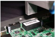
Specialty Tamp Alternative For situations where very small labels need to be applied, such as circuit board applications, the PA1200 supports custom Tamp sizes, which will permit labels as small as .20" wide x .20" high.
