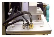
**Tamp / Blow Alternative-**For those special jobs where a Tamp Applicator isn't appropriate, as with concave or convex objects, the Tharo PA2000tb will do the trick! The tamp pad stops between  $\frac{1}{2}$ " and 2" from the product and the label is blown on.
