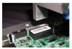
**Specialty Tamp Alternative-**For situations where very small labels need to be applied, as with circuit board applications, the PA2000 supports custom tamp sizes that will permit labels as small as .20" wide x .20" high.
