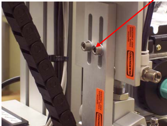
Loosen these bolts to adjust the angle.
