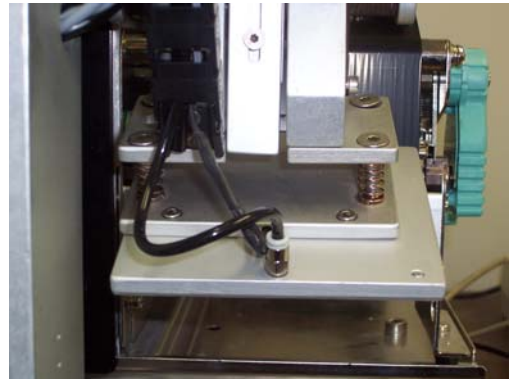
The tamp pad should be aligned with the peel edge.
