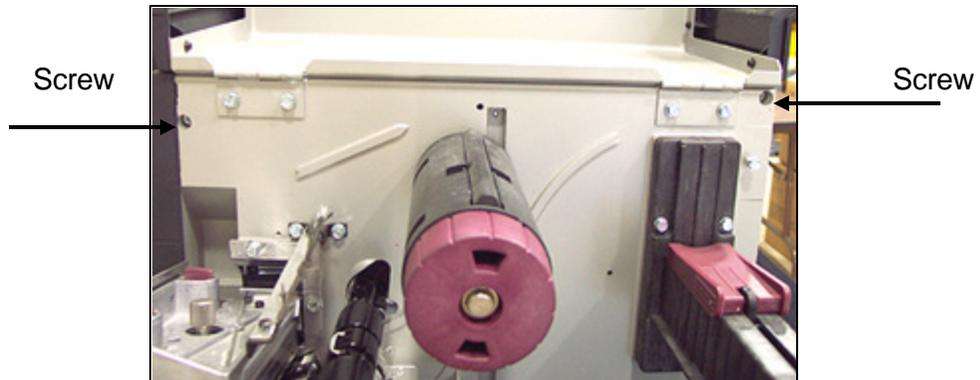
Once the electronics side cover is removed, remove the two remaining screws that are securing the printer to its base.
