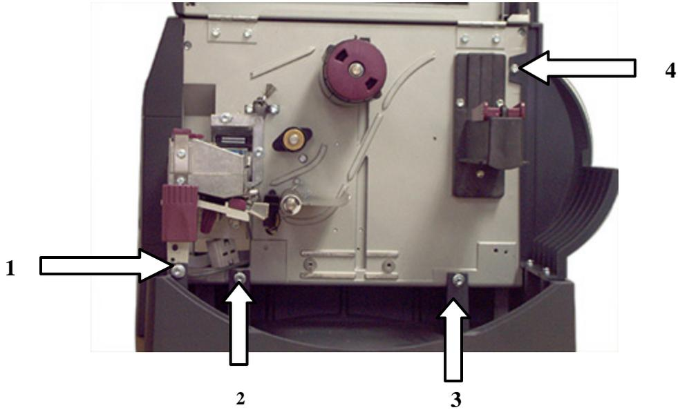
**(Note: You will need to use screws 1,2, and 3 to secure the printer to the base plate!!!)**
